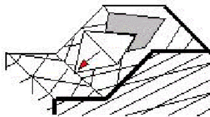
sliding of rock wedges
